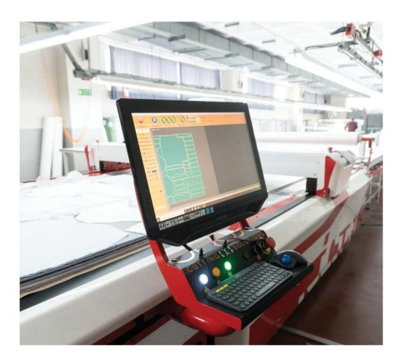
Our manufacturing plant utilizes the latest technology to prepare and cut fabric for production. We have  $iCUT^{\circledast}$  cutting machines, fabric laying machines, and mechanical tables. Using the latest technology allows ERTEN® a **cutting capacity of 10,000 pieces per day**. The sensitivity of the machines can identify different fabric types and adjust accordingly to ensure clean, accurate cuts with millimetric sensitivity and accuracy every time.
